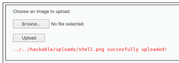
Figure 5.4: The backdoored PNG file successfully uploaded to the target application
