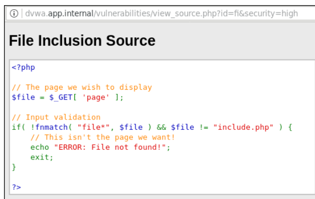
Figure 5.5: File inclusion vulnerability source code
